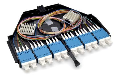
NEXCONEC NGX SPLICING cassettes are designed for splicing up to 24F in a cassette. The NGX cassettes are designed to easily plug into NEXCONEC NGX 1U 6 slot panel and each chassis can populate up to 144F with LC and 72F with SC. The cassettes are preloaded with adaptors and pigtails supplied with splicing accessories.
